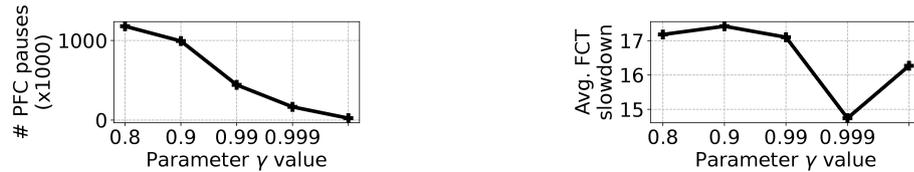
Figure 5.13: As the parameter  $\gamma$  value approaches 1, REVERIE becomes oblivious to the changes in the buffer and drastically reduces the number of PFC pauses. However, beyond a certain value, the lack of PFC pauses negatively impacts FCTs.
